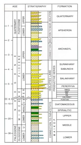
Figure 3. Schematic stratigraphic column for the central South Caspian Basin. Note the break in linear time scales at 6 Ma.
