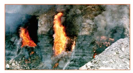
Figure 1. Open-pit mine fire near Dhanbad, Jharia Coalfield, India. Most Jharia fires ignite spontaneously, subsequent to mining. The middle flame is ~7 m (23 ft) high. Source: Daniel B. Sanger, GAI Consultants, Inc., Homestead, Pennsylvania, USA.
