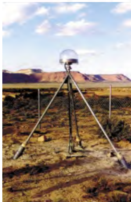
Figure 3. Photograph of Wyatt-design BARGEN monument and GPS antenna at site FRED. Monuments are constructed with one vertical borehole and three slanted boreholes plunging 55° with azimuths of 0°, 120°, and 240°, to a depth of 10 m.
